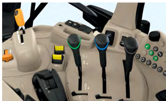
AutoPowr on the right-hand console with mechanical SCVs
