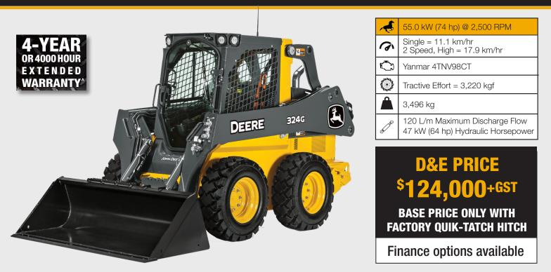
Incorporating many of the same durability and reliability features found on our larger machines, the G-Series skid steers are as tough as they come. Uptime advantages such as rugged Yanmar engines, in-boom hydraulic lines and wiring, large coolers, and extended service intervals help keep downtime down. Plus, a standard automatic shutdown system prevents overheating or low fluids from ruining more than just your day. When you know how they're built, you'll see what they can do.
