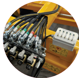
Electro valves for multiple hydraulic operations
