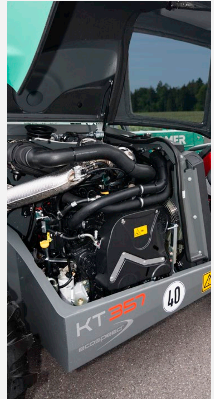
Water-cooled 4-cylinder in-line engine with cooled external exhaust gas return, turbocharging and intercooling.
