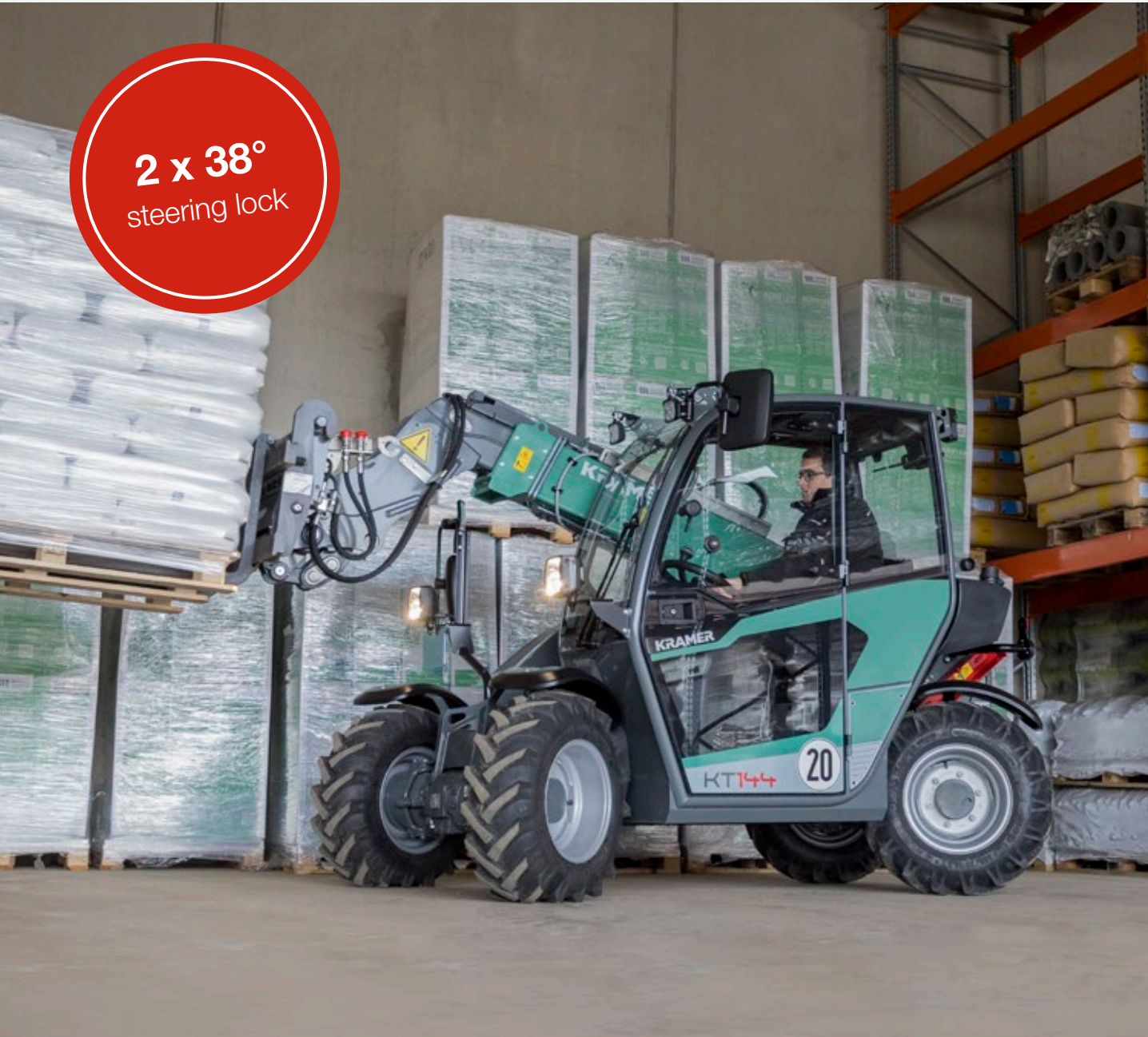
All-wheel steering: particularly manoeuvrable in tight spaces
