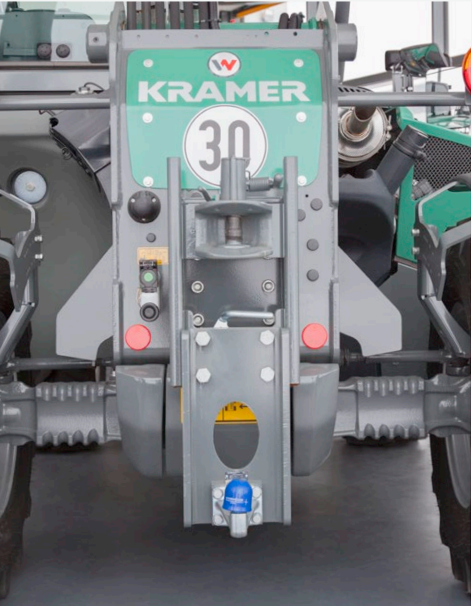
External operating elements (KT276) for the rear power lift and the PTO shaft.
