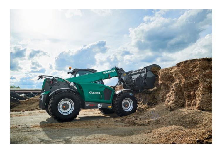
The sturdy telehandler KT557 is designed for extremely demanding tasks. Trailer loads of up to 20 tonnes are no problem. The 156 hp Deutz engine (exhaust emission level V) combined with the standard ecospeedPRO drive system ensure excellent handling capacity. Partly-automated work cycles using the Smart Handling system can significantly increase the mass movements per hour. The multifunctional load stabiliser allows for a gentle application for man and machine.
