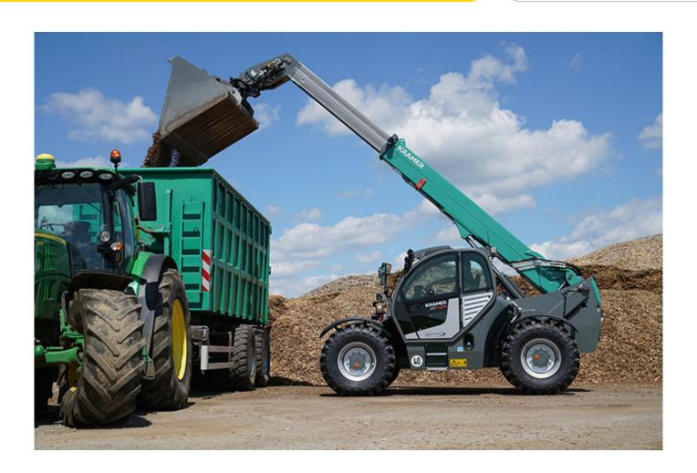
9 m stacking height, a maximum payload of 4.2 t and 40 km/h final speed, as well as fast load processes are easy with the Kramer telehandler KT429 thanks to its sensitive load-sensing gear pump. Innovative details such as the 7 inch display, on which all vehicle data can be read, make the work easier. The new Jog Dial is operated intuitively and can, for example, set the work hydraulics.
