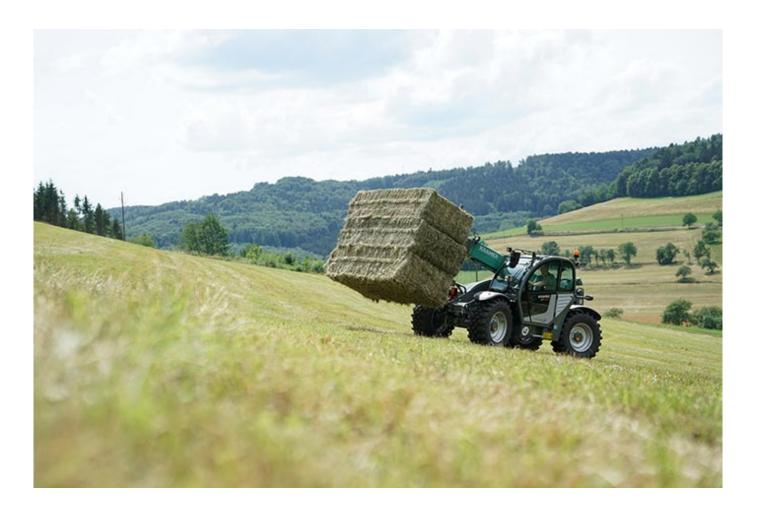
4.0 t payload and its compact dimensions of 2.30 m width and 2.31 m height make the KT407 a true all-rounder on any agricultural operation. The many options allow this telehandler to adapt to the most diverse application areas in agriculture. Technically speaking, the KT407 convinces with a 136 hp-strong Deutz 3.6 L4 engine and its high hydraulic performance of 140 l/min.
