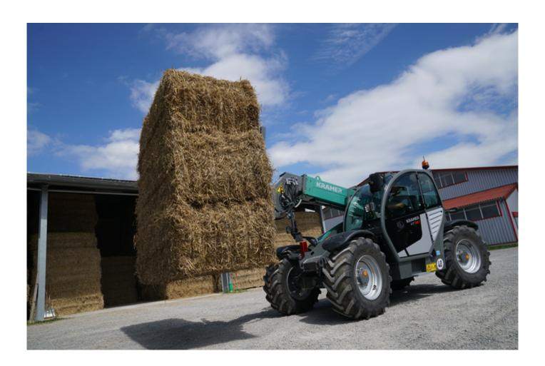
The Kramer KT357 is a manoeuvrable, compact and powerful telehandler, which was designed for agricultural work. The maximum lift capacity of 3.5 tonnes and stacking height of 7 metres provides outstanding versatility for all farm and loading activities. The overlapping area between the inner and outer arm > 1 m is another example of its sturdy design. Its 136 hp engine as well as the standard load-sensing hydraulic system provide for performance that you need.
