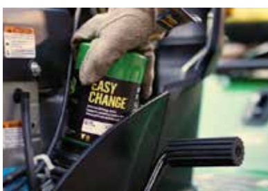
John Deere Easy Change 30 Second Oil Change System *on selected models
