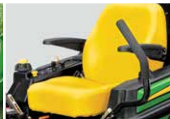
New seat slide. Features fore and aft dampening when used with both the base deluxe comfort seat and the isolation seat option. Experience enhanced ride quality and reduced rider fatigue.
