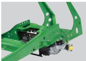
Heavy-duty C-channel frame. Built like a truck, for greater durability.
