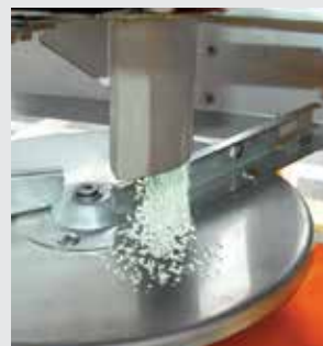
Setting gauge corresponding to the spreading charts for highly accurate fertilization
