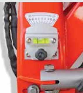
Tilt regulator for late spreading
