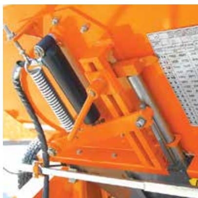
Hydraulic regulation of fertilizer quantity-control
