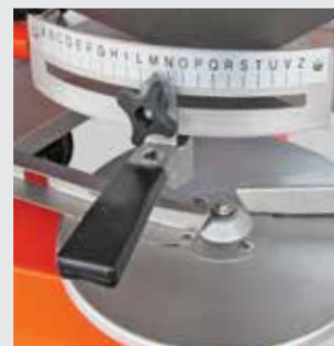
Setting gauge corresponding to the spreading charts for highly accurate fertilization
