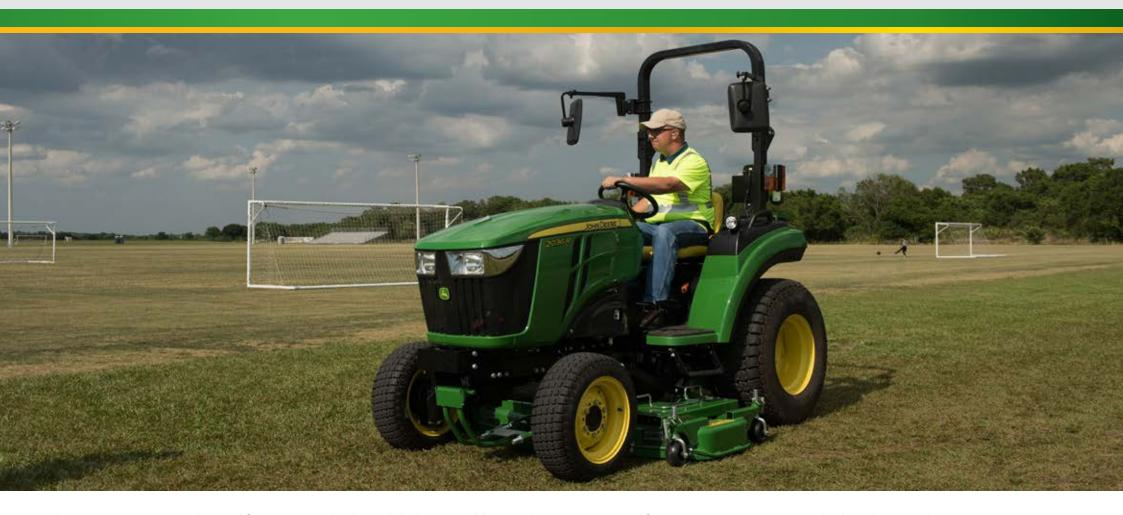
The 2R Series Tractors are designed for operators who demand the best available performance, yet desire a relatively compact machine. With engine power of 27.3 kW (36.6 hp), the 2036R will exceed operator expectations for power across the expanse of Category 1 implements mounted in the rear and/or front of the tractor.
