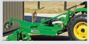
To quickly change implements with the iMatch Quick-Hitch, you simply back in, hydraulically lift the unit and secure the latches.
