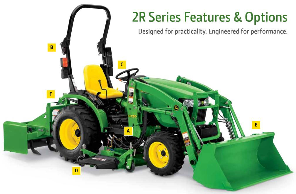
**A.** 2-speed, 2-pedal hydrostatic transmission with cruise control means simple operation, even for inexperienced drivers.
