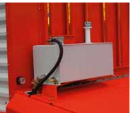
On-board hydraulics for cross conveyor belt
