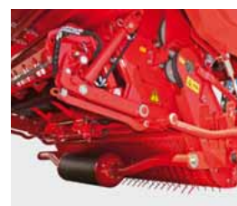
Additional tracking roller for pick-up
