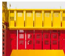
Hydraulic folding automatic loading flap
