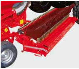
Knife bank swings out alongside wagon
