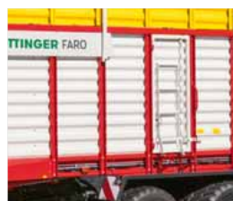
Access door with ladder
