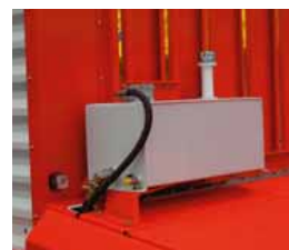
On-board hydraulics for cross conveyor belt
